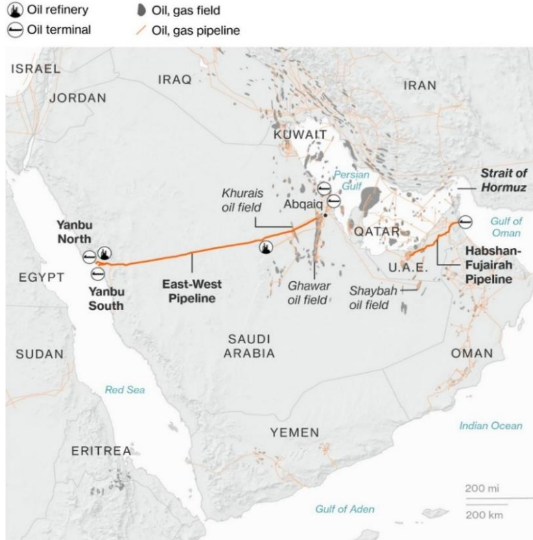
Figure 3 Pipelines bypassing the Strait of Hormuz, Source: CIA, US Department of Energy
